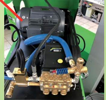
TEFC electric motor, General industrial pump, Phoenix switch
